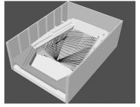
above the heads of the audience which can render the cellos inaudible. We have found that by tilting the side walls inwards, the sound will propagate from sufficiently above audience head-height to avoid this effect. In the unique design of Omsk, we have employed both reverse-fan shaping and tilted walls to enhance the strength of the early lateral sound. Although Omsk is the first concert hall to have these features, its success ensures that it will not be the last
